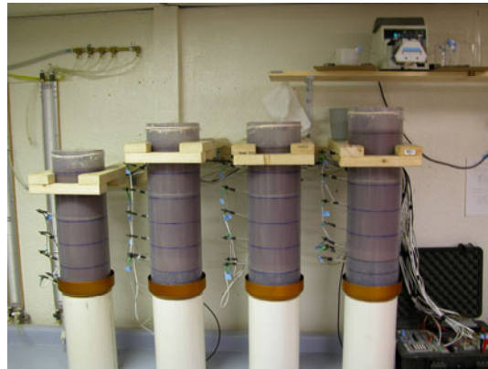
Figure 3. Column tests to simulate capillary barriers, Albuquerque, NM.
