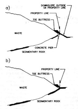
Figure 1: Typical profiles of the toe buttress at the OII Superfund Landfill.
