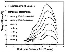
Figure 4. Estimated geogrid strains induced by seismic loads.
