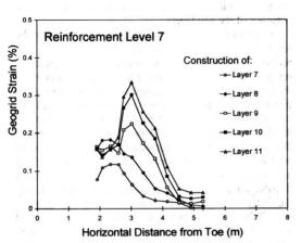
Figure 3. Estimated geogrid strains induced by increasing differential settlements.
