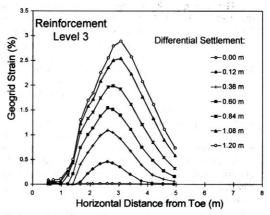
Figure 2. Estimated geogrid strains induced during construction.
