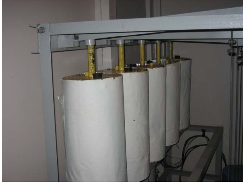
Figure 7. View of incubation cells at GSI, maintained at various constant temperatures.
