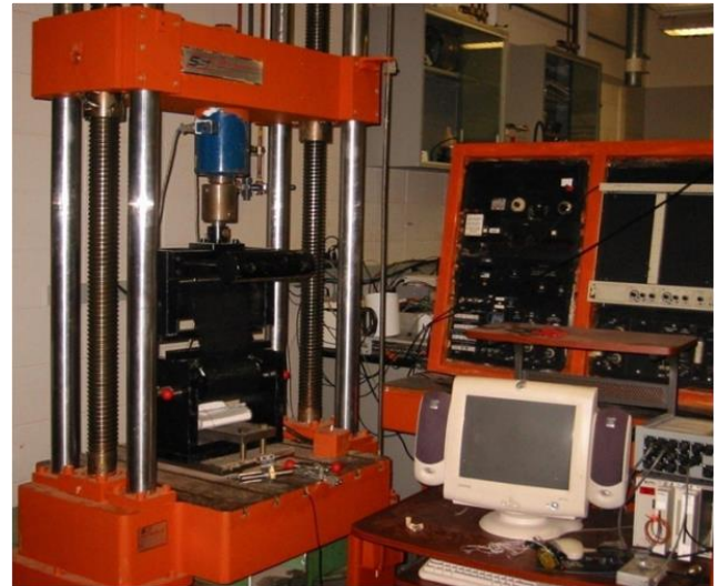
Figure 8: Wide-width tensile test conducted with roller grips at the University of Texas at Austin
