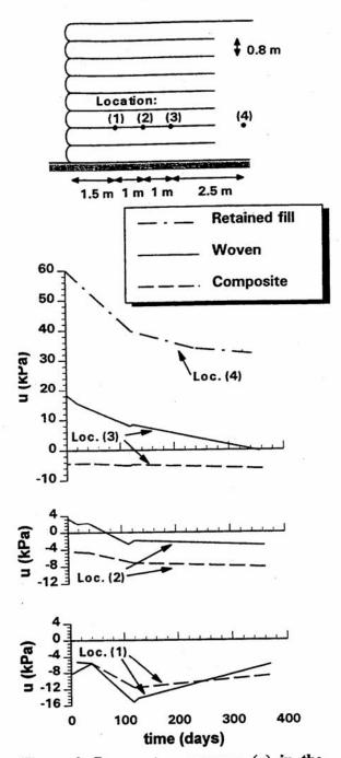
Figure 2. Pore water pressures (u) in the Rouen reinforced wall, along a woven and a nonwoven/geogrid composite, within a silty backfill (redrawn after Perrier et al., 1986)
