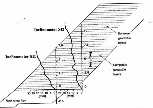
Figure 5. Horizontal deflections obtained from inclinometers within the reinforced fill
