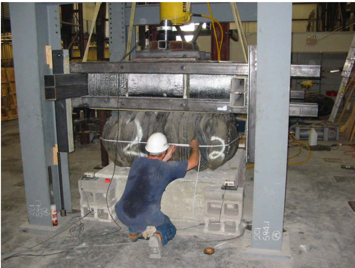
Figure 6: Circumferential measurements. Outriggers mitigated rotation problem.
