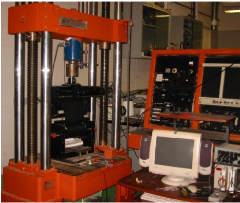
Figure 14: Wide-width tensile test conducted with roller grips at the University of Texas at Austin
