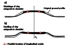
Figure 1: Mechanism of longitudinal crack development on pavements over expansive clays
