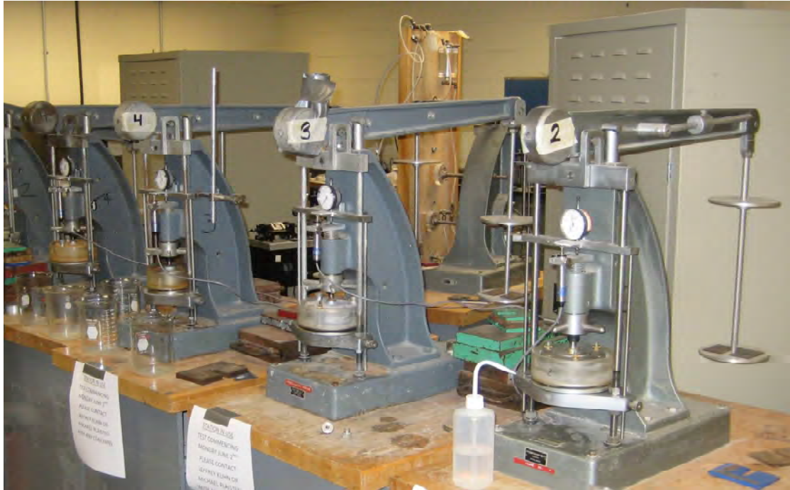
Figure 3.4: Free-swell testing setup
