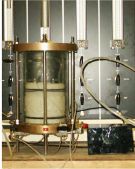
Figure 3.10: Flexible-wall hydraulic conductivity test
