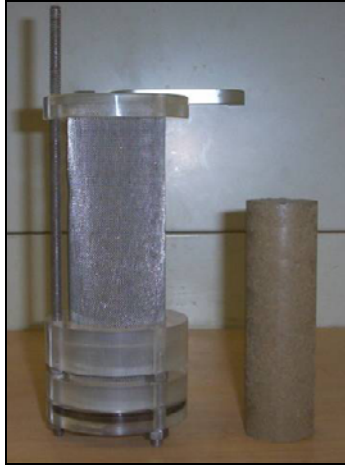
Figure 5.1: Cyclic wetting and drying specimen holder and compacted specimen
