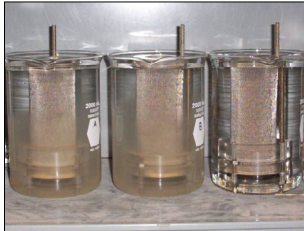
Figure 5.2: Submerged specimens during the wetting portion of cyclic wetting and drying test series
