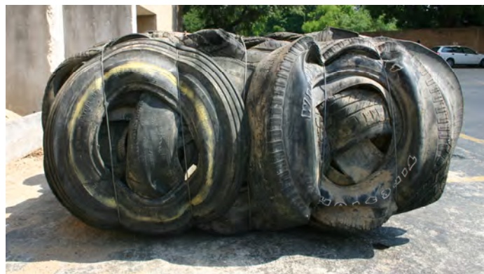
Figure 3.1 View of one of the tire bales used in the experimental testing program
