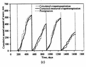
Figure 8. Hydrus-1D results: (a) Moisture content at three depths (277 mm, 678 mm and 1080 mm); (b) Surface evaporation and root flux (transpiration); (c) Comparison between calculated and measured evapotranspiration.
