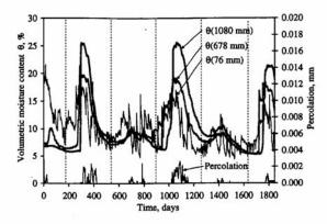
Figure 3. Percolation and volumetric moisture content at three depths (76 mm, 678 mm, and 1080 mm).
