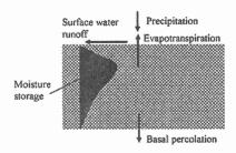
Figure 1. Schematic of an evapotranspirative cover.
