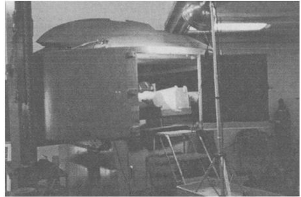
FIG. 3—View of the Schaevitz geotechnical centrifuge.
