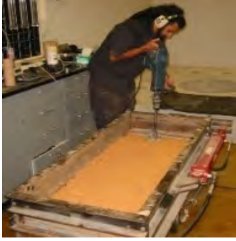
a) Compaction of soil in layers
