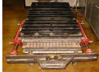
e) Rubber membrane and steel plates over compacted soil
