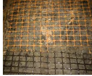
b) Tensile mode of failure at end of test
