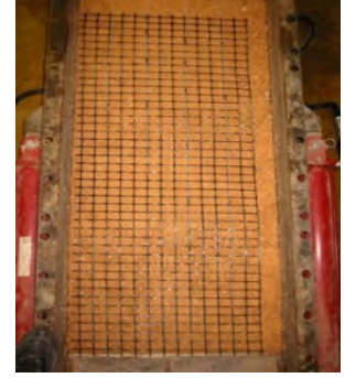
c) Attaching tell tales to the geogrid
