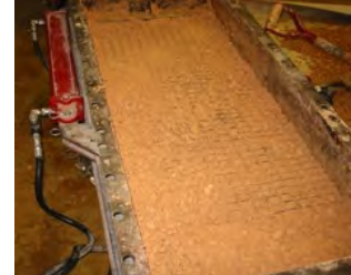
f) Removing soil at end of test and embedded geogrid
