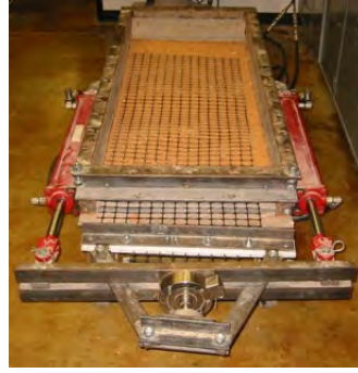
b) Placement of geogrid at end of second layer
