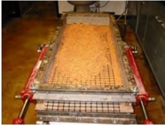
d) Soil compaction on top of the clamped geogrid
