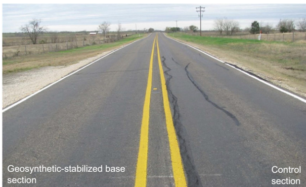
Figure 26. View of road conditions of a control section (right) and a geosynthetic-stabilized base section (left) from 2011 condition survey conducted in FM2 test sections (Case Study E)
