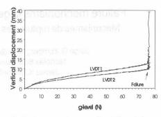
Figure 3. Settlements at the crest of a reinforced slope model
