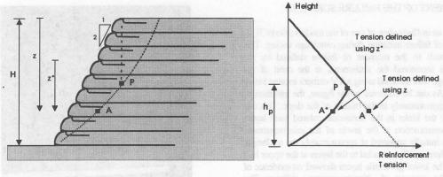
Figure 8. Reinforcement force distribution with depth for reinforced soil slopes
