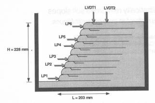
Figure 1. Typical centrifuge model
