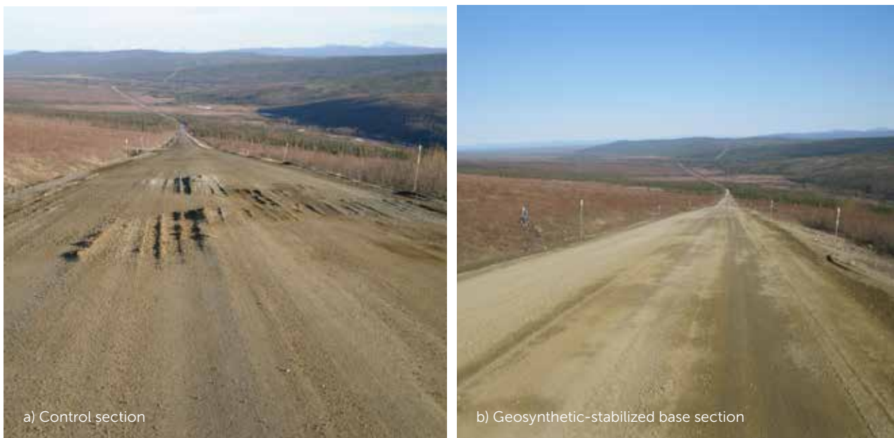
Figure 6. Performance of wicking fabric at Beaver Slide test section on Dalton Highway: a) Before treatment (May 2010), and b) After treatment (May 2011).
