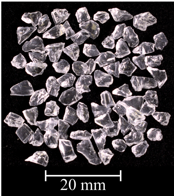
Fig. 2. Fused quartz particles tested in this study.
