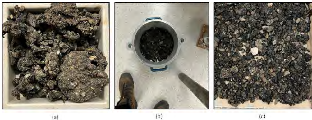
Figure 4. (a) GRAP sample collected from the stockpile; (b) GRAP crushing in the laboratory; and (c) Crushed GRAP sample.
