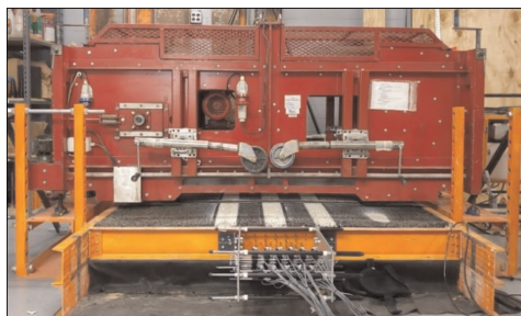
Figure 3. Model Mobile Load Simulator (MLS11) trafficking the pavement test section.
