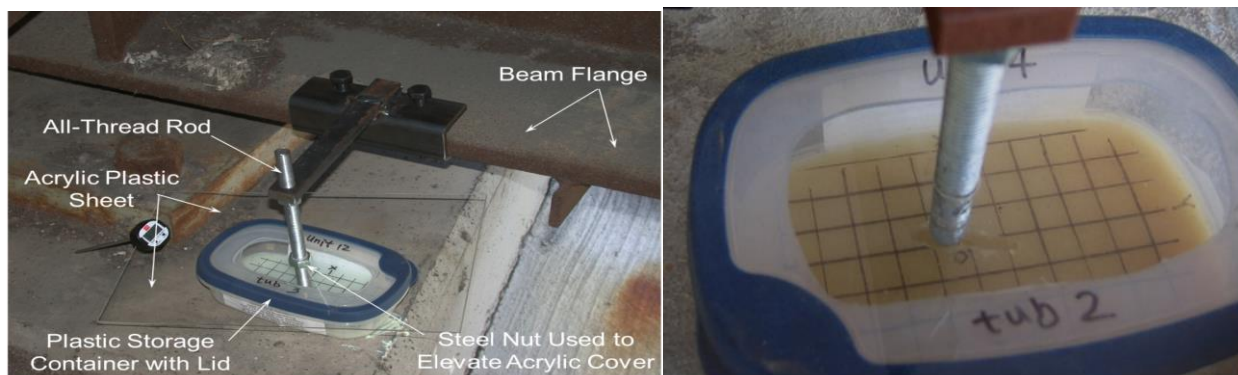
Figure 7.3: Wax trace box for simple deformational measurement (Chen et al., 2009).
