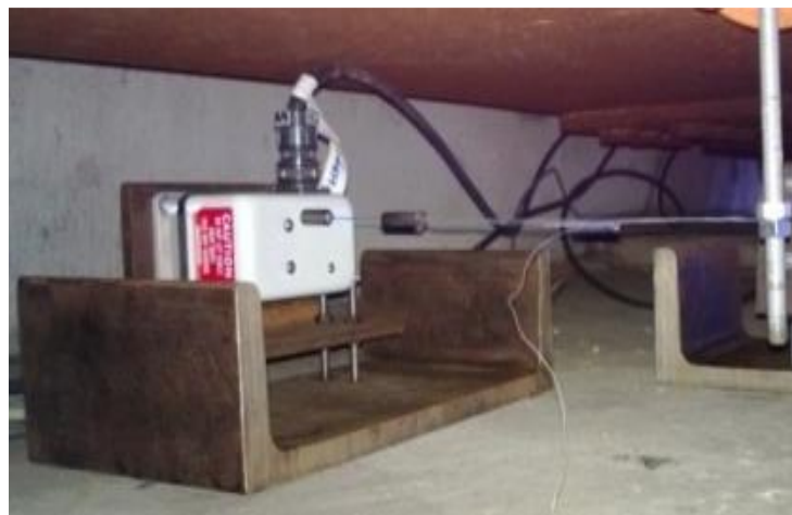
Figure 7.2: Linear potentiometer (string potentiometer) for measuring displacements.
