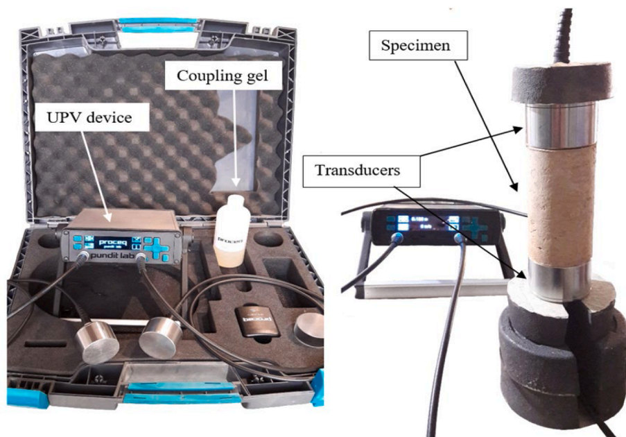
Fig. 4. UPV testing device and view of specimen during testing.
