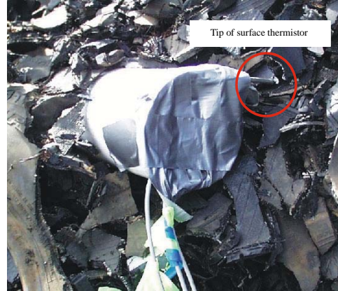
Photo A-26: Detail of Thermistor at the Surface of the Large Tire Shred-Only Stockpile
