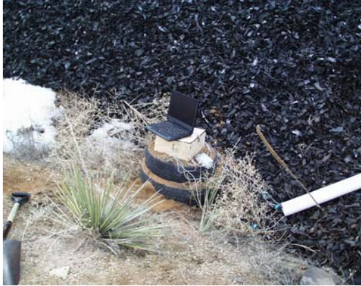
Photo A-31: Detail of Laptop, Data logger and Wiring from the Large Tire Shred-Only Stockpile
