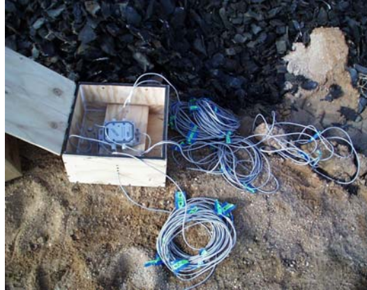
Photo A-32: Data Acquisition Device (HOBO Data logger) for the Large Tire Shred-Only Stockpile
