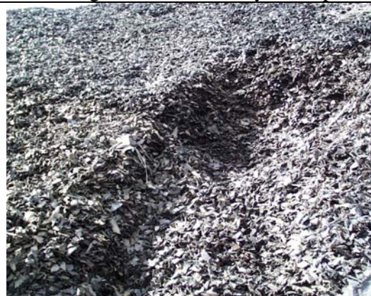
Photo A-30: Closure of the Ditch Excavated for Installation of Instrumentation in the Large Tire Shred-Only Stockpile
