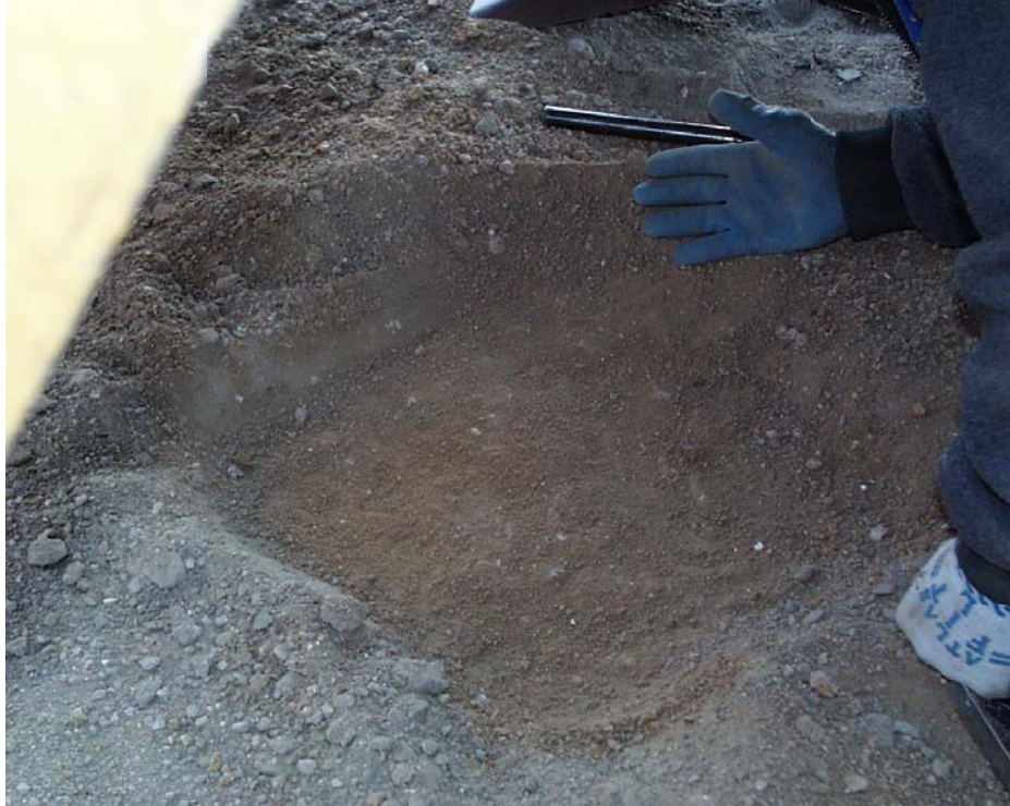
Figure 36: Location of plate-load test, after excavation by hand
