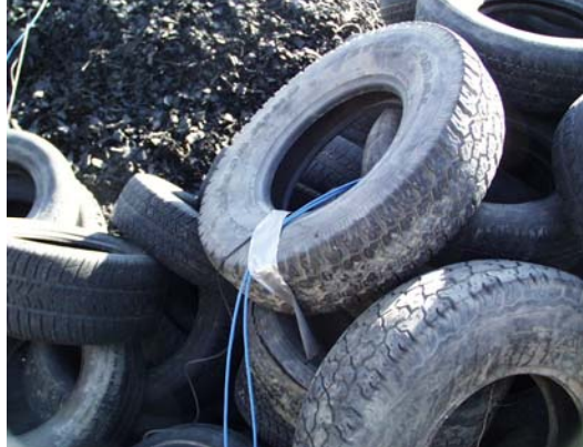
Photo A-18: View of Whole Tire Stockpile with Instrumentation
