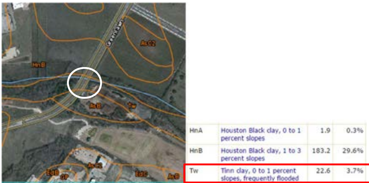
Figure 4.7: Soil Survey Map and Table at Site 2 (USDA 2013)
