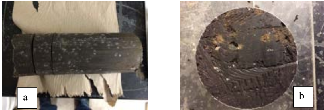
Figure 5.5: B-8 Samples tested at In-Situ (a) and Moisture Adjusted (b) Conditions
