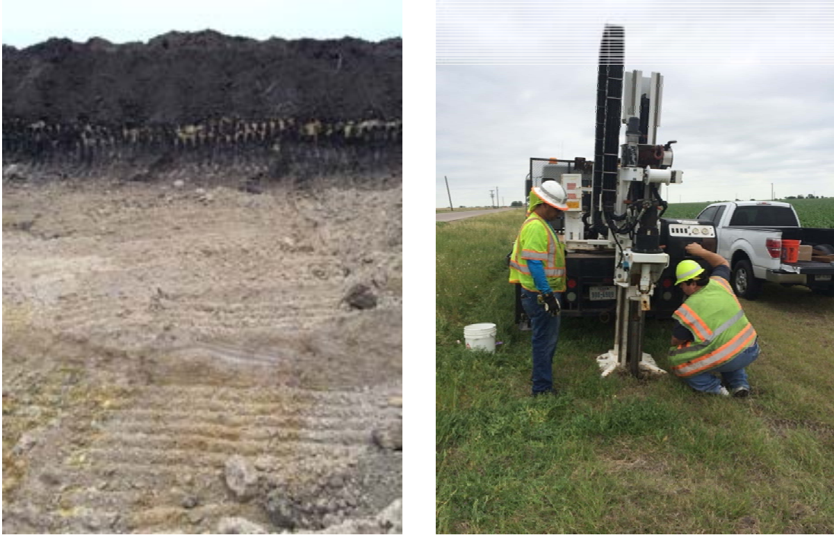
Figure 2.10: Soil Stratigraphy at the Excavation Pit (left, a) and Shelby Tube Sampling at Intersection (right, b)
