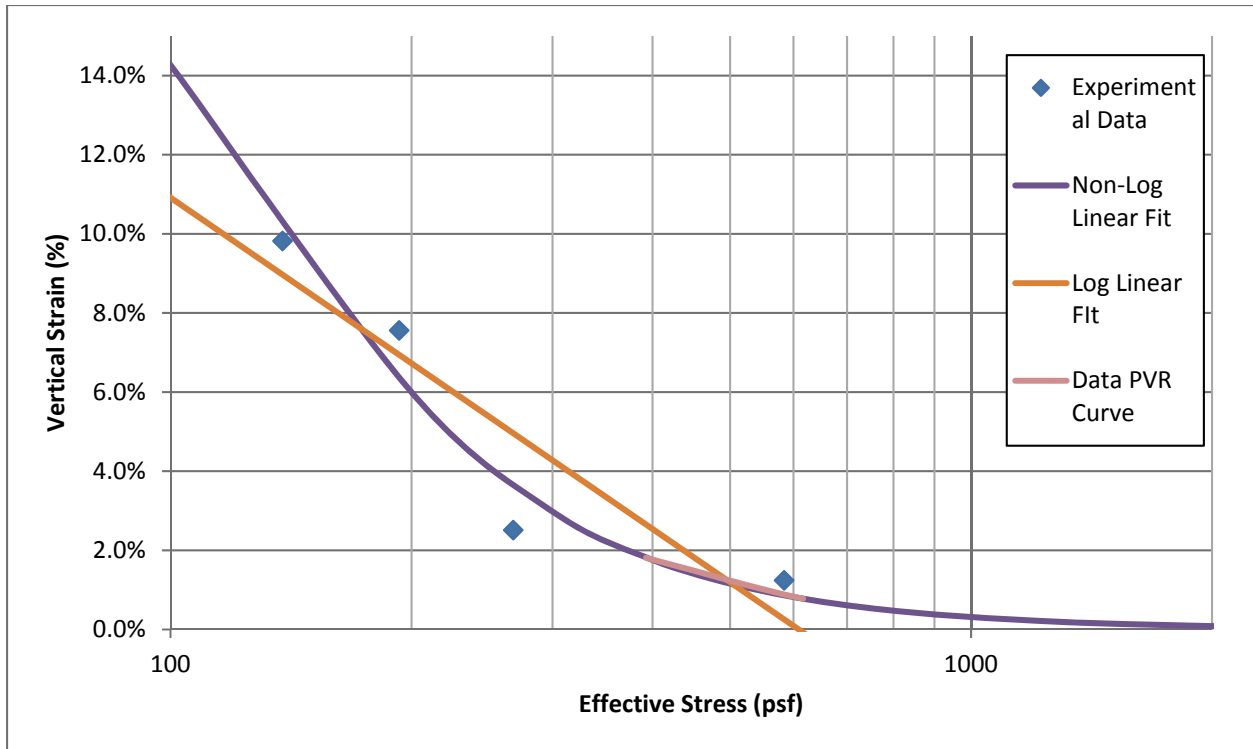
Figure 5.7: Stress-Swell Curves for Bulk Samples from Kelly Lane
