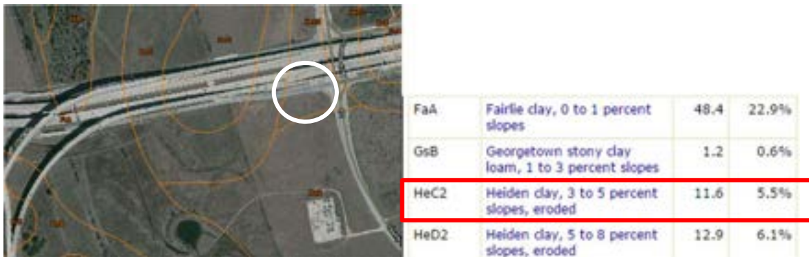
Figure 4.20: Soil Survey Map and Table at Site 6 (USDA 2013)
