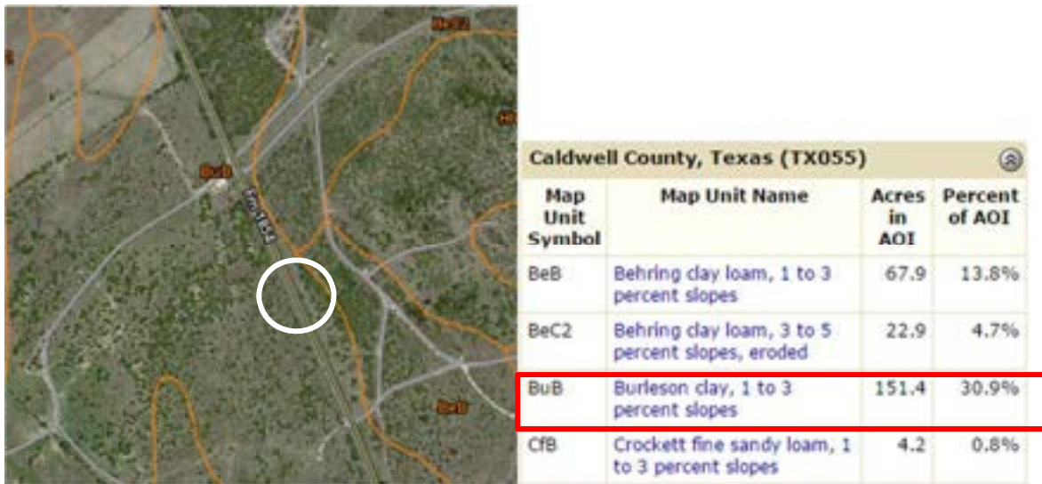
Figure 4.55: Soil Survey Map and Table at Site 15 (USDA 2013)
