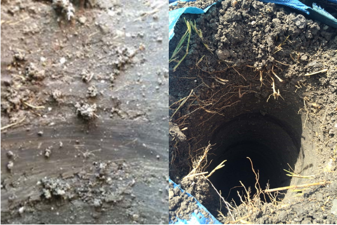
Figure 4.30: Augured Hole and Soil Samples from SH 95
