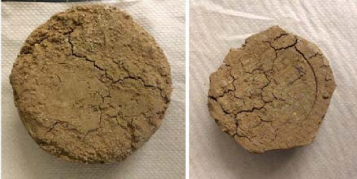
Figure 3.4: Examples of desiccation cracks in moisture conditioned soil specimens formed by excessive moisture-loss and caused by unstable humidity and temperatures during drying (Armstrong, 2014).
