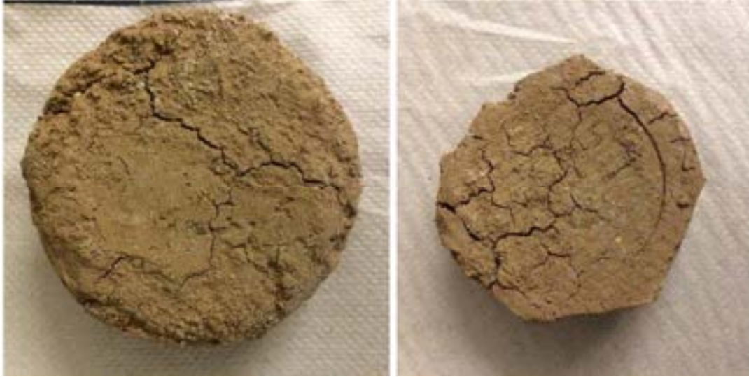
Figure 2.4: Shrinkage Cracks formed from rapid drying.
