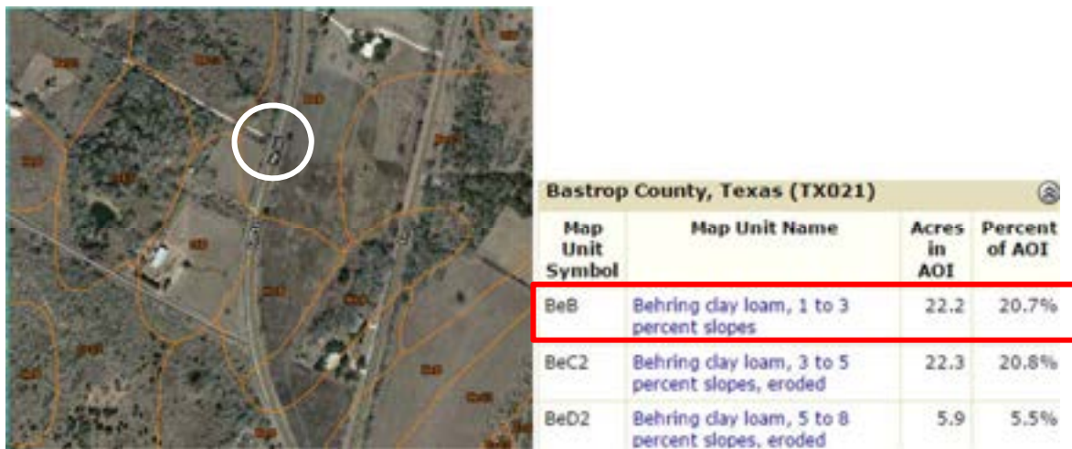
Figure 4.40: Soil Survey Map and Table at Site 11 (USDA 2013)
