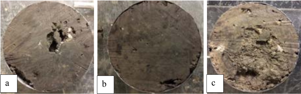
Figure 5.37: B-20 Samples at In-situ (a,b) and Moisture Adjusted (c) Conditions
