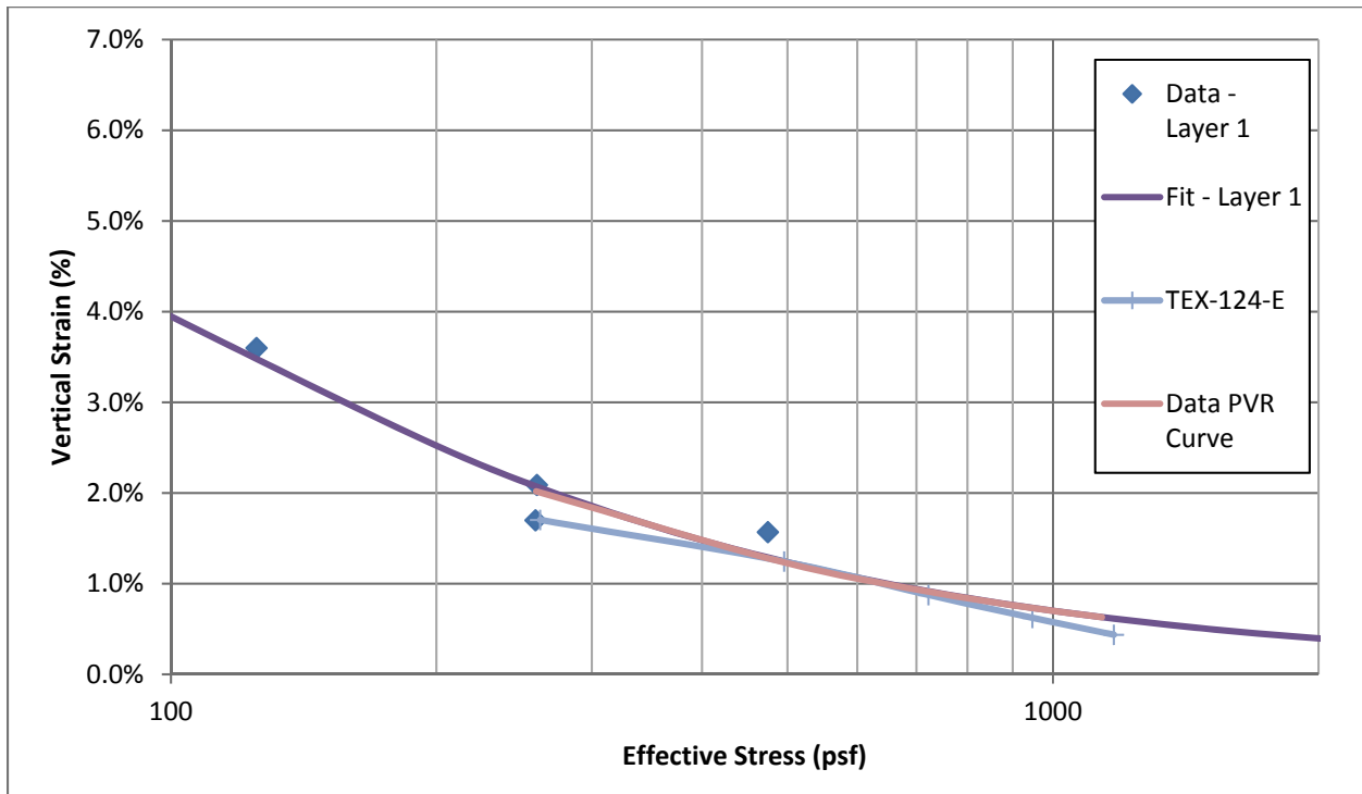
Figure 4.84: Comparison of Swelling Curves from Centrifuge Data and Tex-124-E for Site 2
