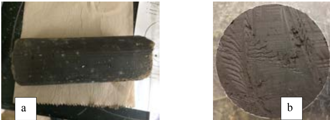
Figure 5.31: B-18 Samples at In-situ (a) and Moisture Adjusted (b) Conditions
