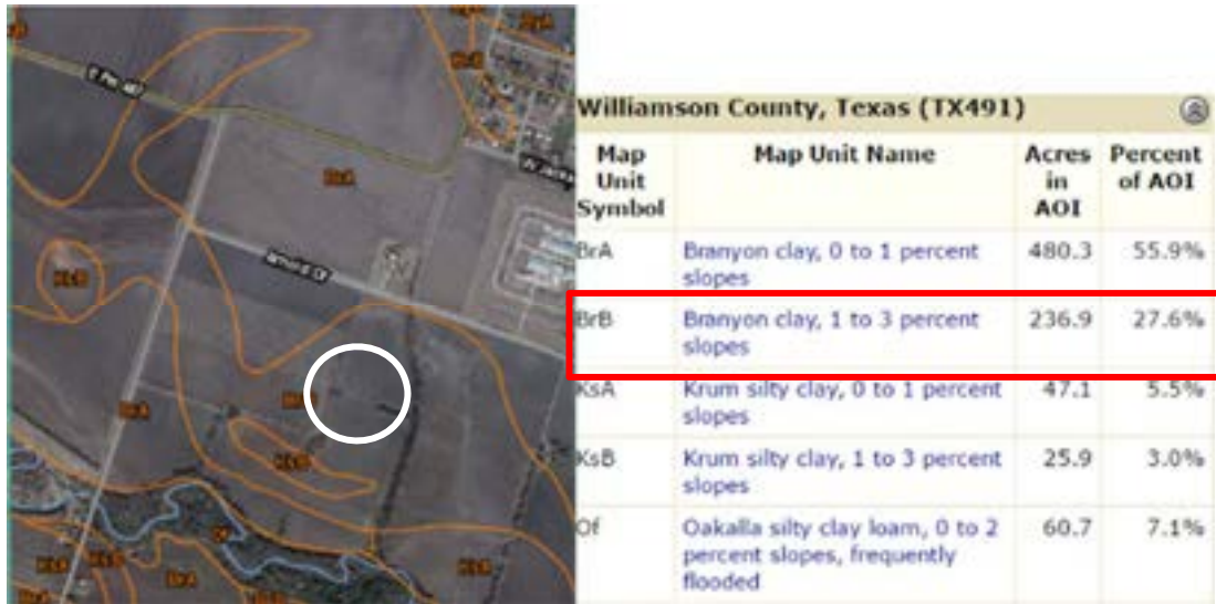
Figure 4.78: Soil Survey Map and Table at Site 19 (USDA 2013)
