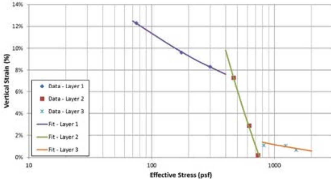
Figure 3.3: An example of a series of stress-swell curves for a profile of three distinct expansive soil units, plotted within the range of stresses expected for each layer.
