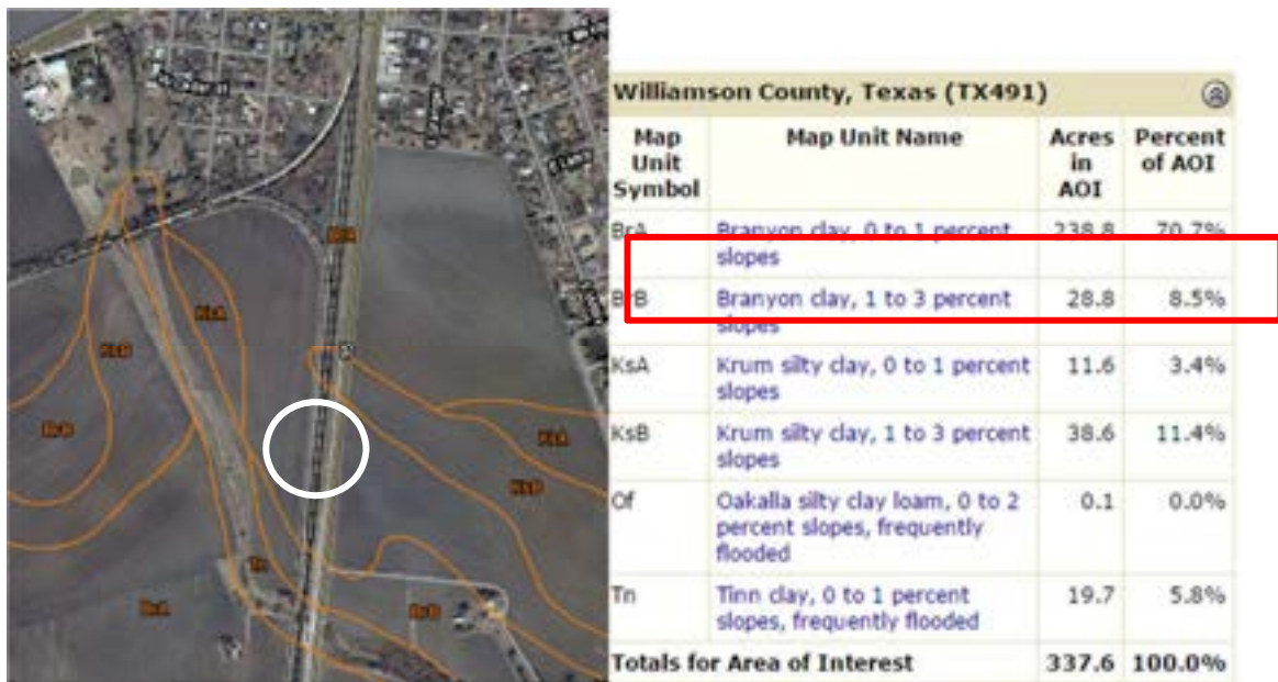
Figure 4.32: Soil Survey Map and Table at Site 9 (USDA 2013)
