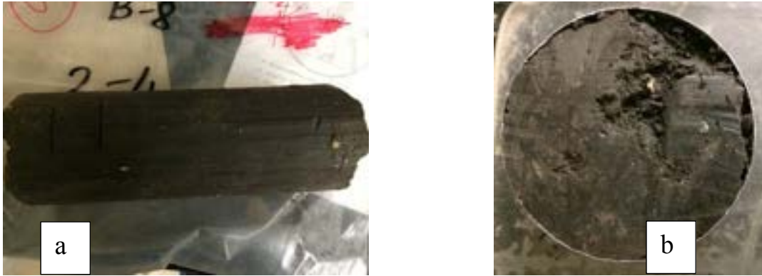
Figure 5.20: B-15 Samples at In-situ (a) and Moisture Adjusted (b) Conditions
