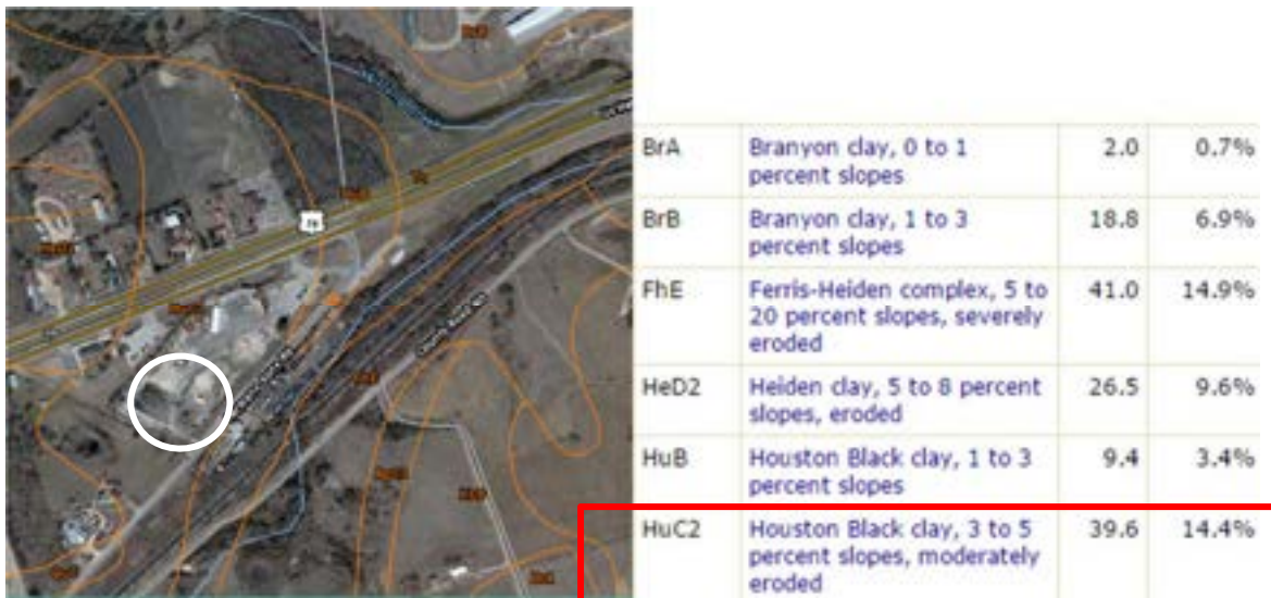
Figure 4.36: Soil Survey Map and Table at Site 10 (USDA 2013)
